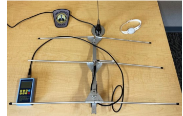
An antenna and tracking device used by Chelmsford Police as part of the SafetyNet program.
